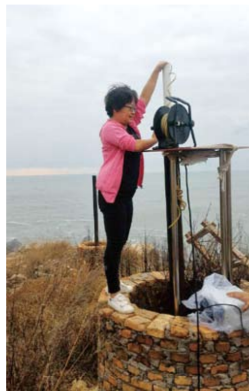
Engineer Qing Li sampling in the D-SMART underground water monitoring well.
